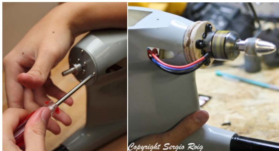
Figure 15.1.1 Motor mount before and after enforcement
