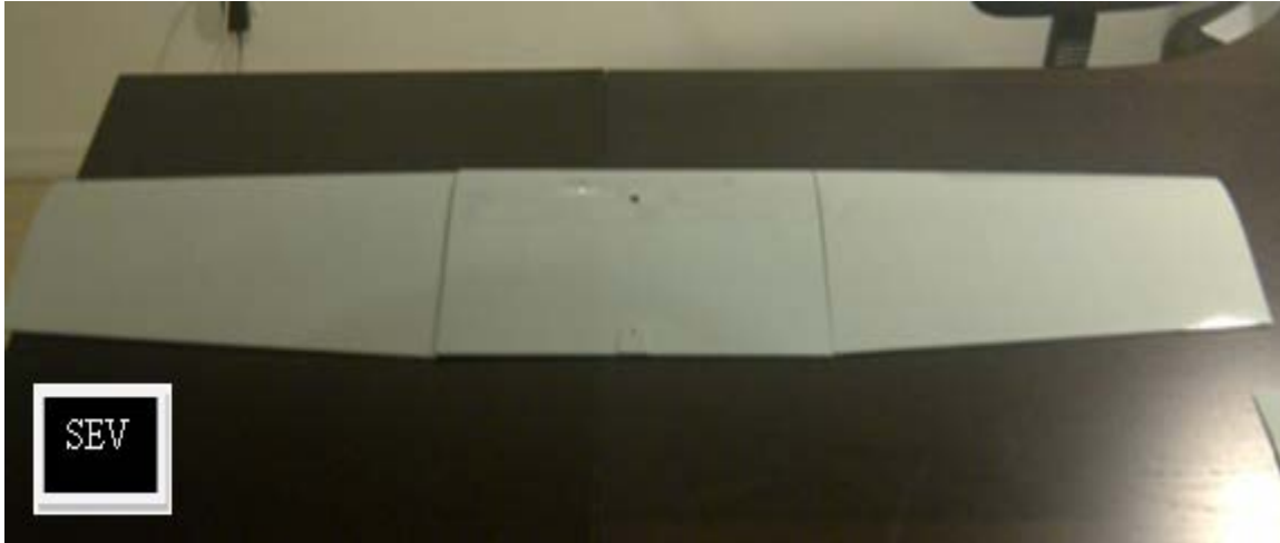
Figure 12.1.4 - Main wing of the RQ-11
